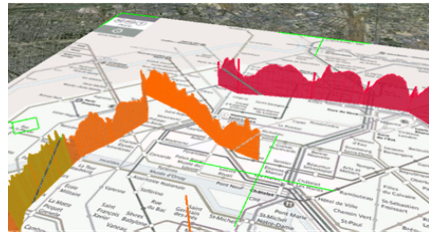
Fig.2 - Noise map of two subway lines (indoor location) reconstructed thanks to the geo-tagging feature in the mobile sensing application
